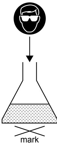
10.0 cm<sup>3</sup> of 2.00 mol dm<sup>-3</sup> hydrochloric acid was added to a 50.0 cm<sup>3</sup> solution of sodium thiosulfate at temperature, T<sub>1</sub>. Students measured the time taken for the mark to be no longer visible to the naked eye. The experiment was repeated at different concentrations of sodium thiosulfate.
